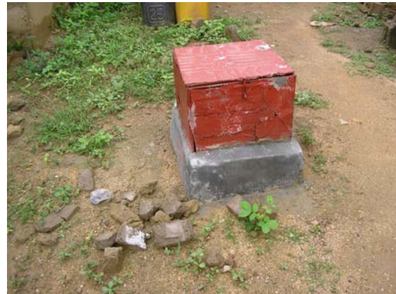
Once the borehole pipings are installed, the hole is sealed tight.
